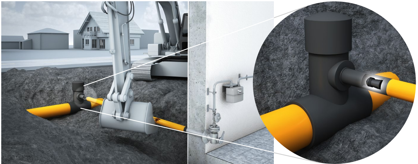
Fig. 1: Excavator damage to service line (SL)
